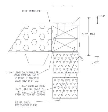
GS SERIES ( GRAVEL-STOP STANDARD ) GRAVEL STOPS ARE AVAILABLE IN VARIOUS METALS. THEY ARE ES-1 TESTED IN 24 GA. STEEL AND .040 ALUMINUM. MAXI-MUM TESTED FACE SIZE IS 8". CALL ULTRA SEAM FOR DETAILS.
