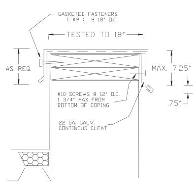
SC SERIES (STANDARD STYLE) COPINGS ARE AVAILABLE IN VARIOUS METALS. THEY ARE ES-1 TESTED IN 24 GA. STEEL AND .040 ALUMINUM. MAXIMUM TESTED FACE SIZE IS 8". CALL ULTRA SEAM FOR DETAILS.
