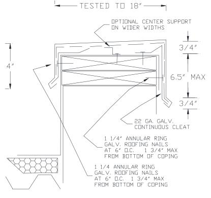
SL SERIES (SNAP LOCK) COPINGS ARE AVAILABLE IN VARIOUS METALS. THEY ARE ES-1 TESTED IN 24 GA. STEEL AND .040 ALUMINUM. MAXIMUM TESTED FACE SIZE IS 8". CALL ULTRA SEAM FOR DETAILS.
