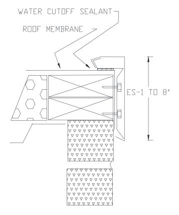
UE SERIES ( ULTRA EDGE ) EDGINGS ARE AVAILABLE IN VARIOUS METALS. THEY ARE ES-1 TESTED IN 24 GA. STEEL AND .040 ALUMINUM. MAXIMUM TESTED FACE SIZE IS 8". CALL ULTRA SEAM FOR DETAILS.
